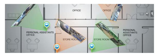
**Immersion mode** represents a leap beyond the standard functionality of the interactive map. In this mode, semi-transparent video is overlaid above a map which remains partially visible. This allows easily seeing where an object is located and where it is going. For closer correspondence of video renderings to the map, you can match points in the video to points on the map. Then the map in immersion mode will be displayed so that the points in the video and on the map coincide.
